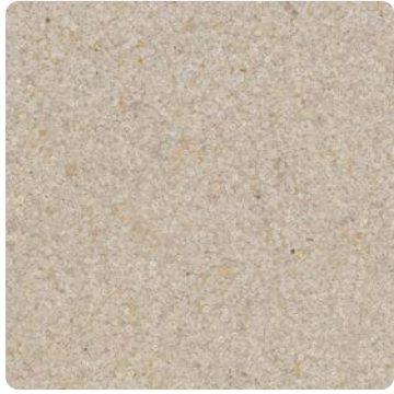
40-S Broadcast (40 Mesh, Spherical)
